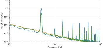
If you encounter EMC noise in the measured signal, which typically arises as peaks in the power spectral density of the measured signals at multiples of the frequency of the electricity supply (50Hz or 60Hz), please check the grounding of your measurement system, see p9. Please also check that you have used shielded cables and connectors from the sensor to the acquisition device.
