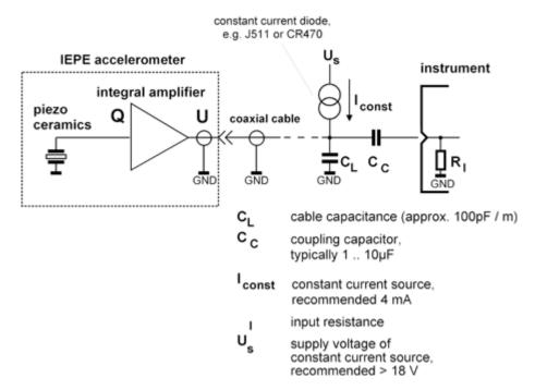
**Warning:** IEPE Dragonfly<sup>®</sup> sensors will not work without the supply current and required dedicated IEPE inputs. IEPE range is specified between 2mA and 20mA. Our sensor work within this range but has been specifically tuned to operate at 4mA. The low cutting frequency of the Dragonfly<sup>®</sup> measured by an IEPE acquisition system depends on two components:
